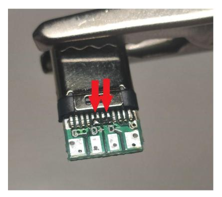
Now solder one end of the RCA cable to ground and the other to D+ and D- (TO BOTH)
